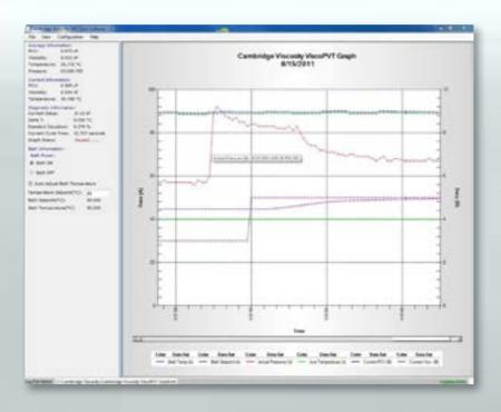
A portable computer integrates timestamped viscosity, pressure, and temperature data into a graphical format for easy analysis and storage. All data can be exported to LIMS or other computers via serial communications. An accessory kit is included with each system to facilitate sample loading, system cleaning, and calibration verification.
